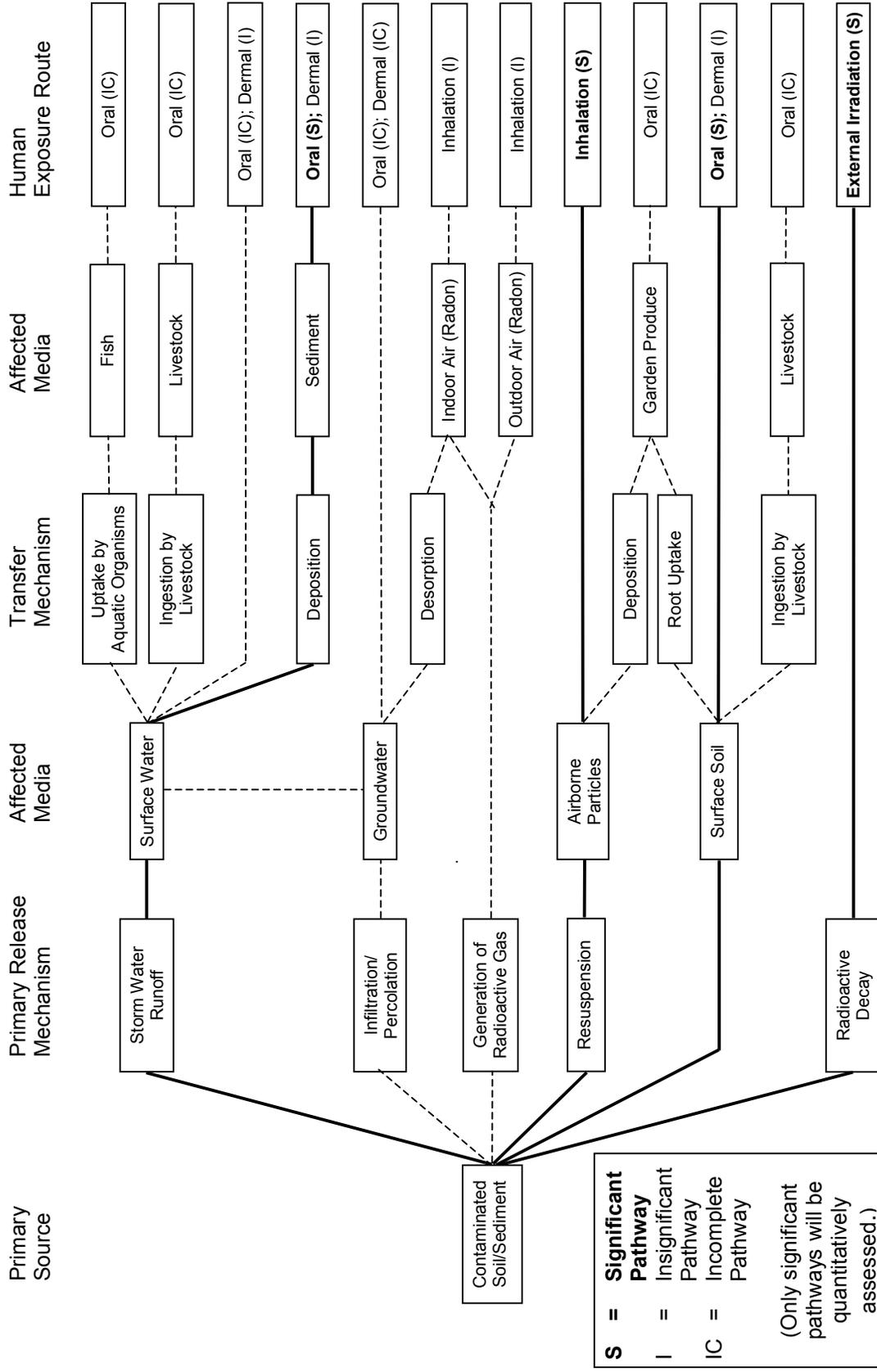
Figure 1. A Conceptual Site Model Developed for Rocky Flats
